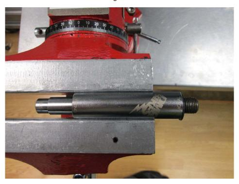
Mount the DMR pedal tool in the vice with the threaded end out.
