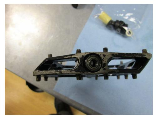
Using the axle you can gently push the old cartridge bearing out the other end, no hammering needed.
