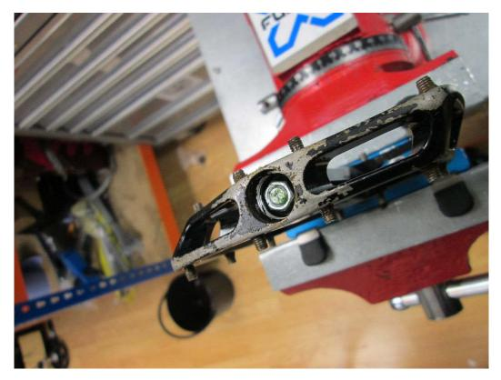
Remove the 6mm Alloy end cap to expose the 9mm nut. \*Magnesium pedals have gold end caps\*
