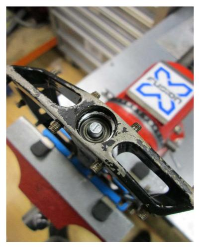
Slide the pedal body onto the axle making sure the axle protrudes through the cartridge bearing.
