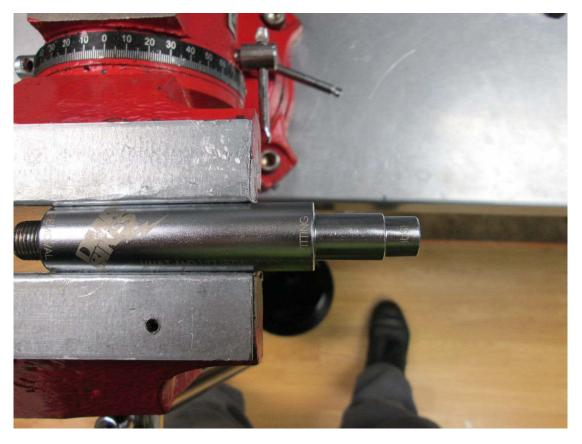
Flip the DMR pedal tool around in the vice so the end marked \*BUSH is sticking out.
