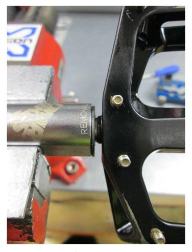
Thread the Pedal body onto the threaded part of the tool whilst applying pressure to engage with the bushing.
