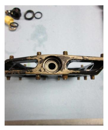
Next, place the cartridge bearing in the pedal flat against the shoulder in the body.
