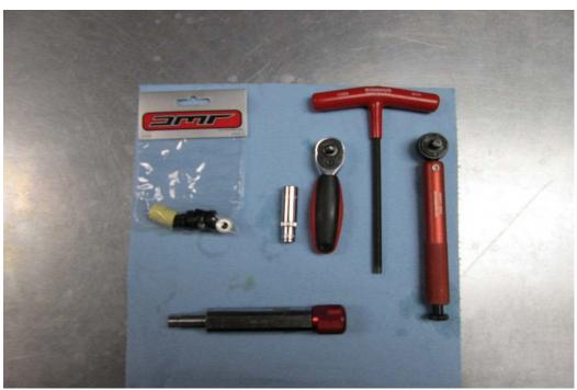
Tools Needed: 6mm Allen Key, DMR Vault & V12 Tool, ¼" Ratchet with 9mm Socket, ¼" Torque Wrench
