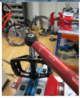
Install the new nut and torque to a maximum of 10Nm then fit the 6mm alloy end cap.
