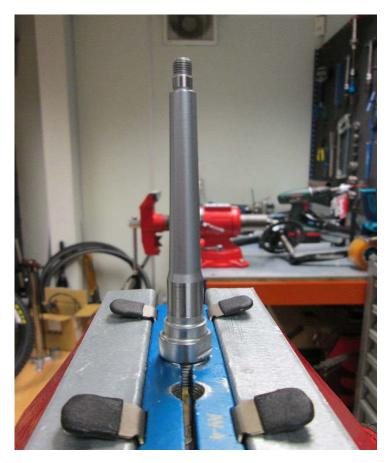
Remove the 2 old rubber seals and clean the axle of any old dirt and grime and inspect for any imperfections on the bearing surfaces.
