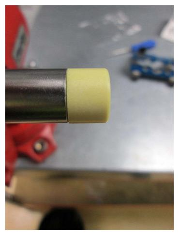
Slide the new bushing onto the tool ready to be pushed into the pedal body. Notice that one end of the bushing has a slight chamfered edge, that enters the pedal first.
